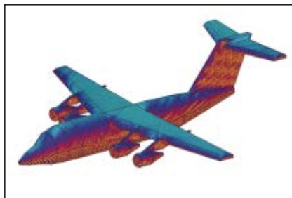
▲ Fig. 5 A surface current plot of an illuminated 120 wavelength long aircraft solved with the new Integral Equation Solver.
